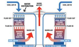
SPRAY PUMPS COOL WATER COLLECTS, IS PUMPED BACK UP CWT Jedair™ Fan driven by CWT Gear Drive Whisper System Whisper System Access Door Both Ends Overflow FLTC-000A
